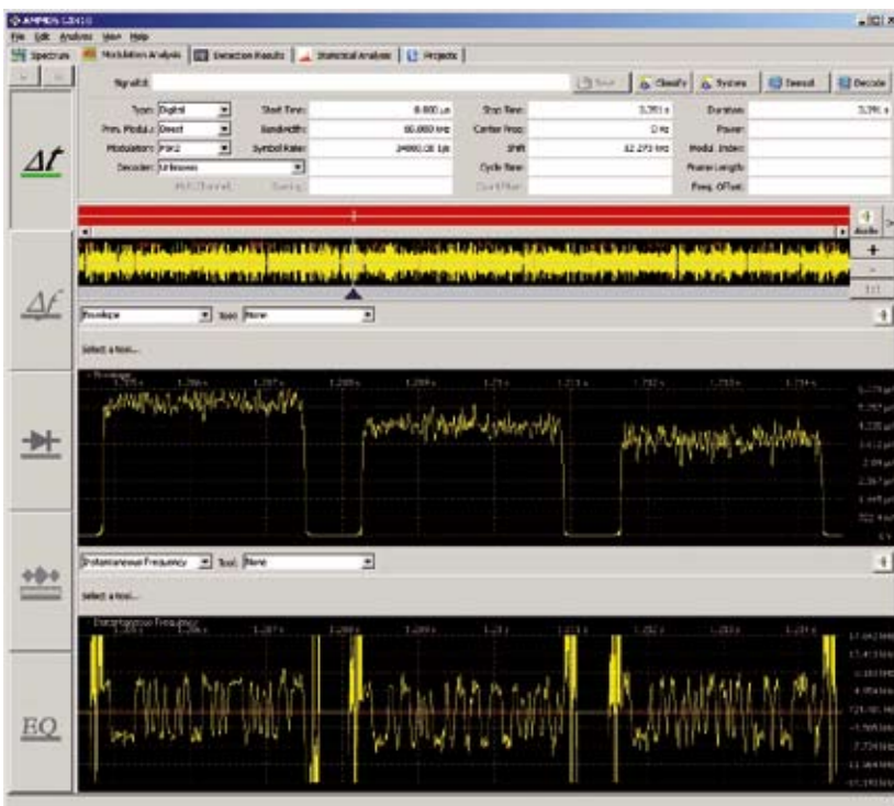
A recombined signal with precisely defined time parameters represented in various ways. Top to bottom: oscilloscope, amplitude versus time, frequency versus time. The time guard period between the short-time emissions and the modulation mode of the short-time emissions (FSK2) are clearly displayed.
