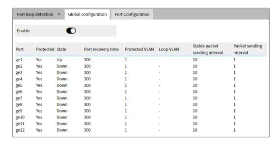
The main element configuration description of global configuration interface:
