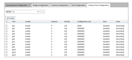
The main element configuration description of instance port configuration interface:
