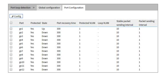
The main element configuration description of port configuration interface:
