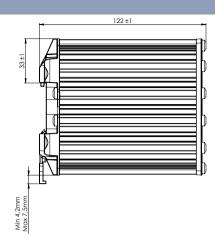
Dimension  $134 \times 100 \times 122 \text{ mm} (5.25 \times 3.93 \times 4.80 \text{ in})$
