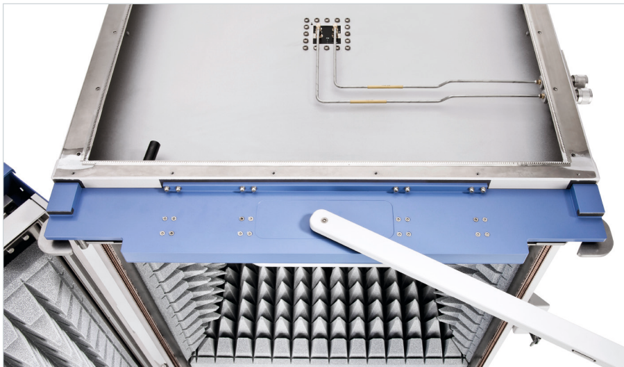
Top compartment for installing RF circuits.
