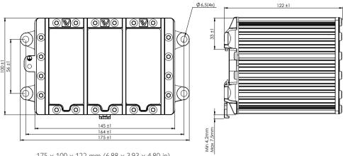
Dimension  $175 \times 100 \times 122 \text{ mm } (6.88 \times 3.93 \times 4.80 \text{ in})$
