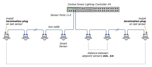
end-to-end Smart Sensor bus length max. 200m total number of Smart Sensors max. 24
