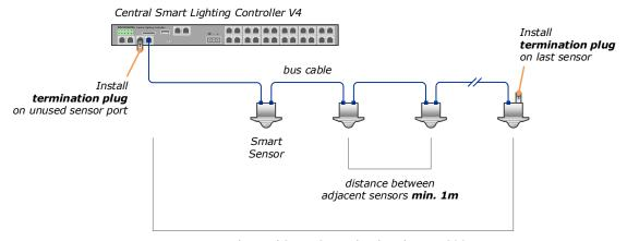
end-to-end Smart Sensor bus length max. 200m total number of Smart Sensors max. 24
