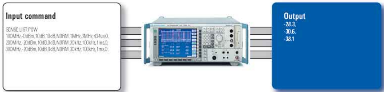
Remote control of R&S FSP via IEC/IEEE bus in list mode cuts down on measurement time
