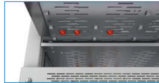
Metal rollers assembled on the withdrawable unit.
