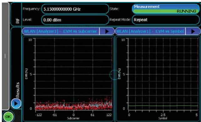
802.11ac 80 MHz VHT MC8 EVM vs. subcarrier and symbol
