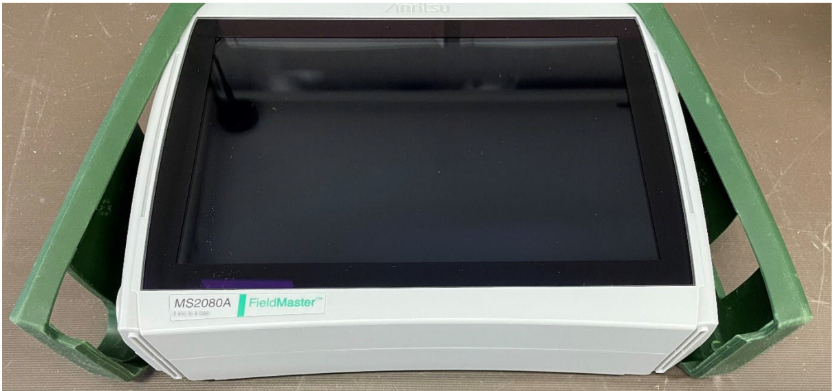
Figure 3-3. Pulling of Side Bumpers
