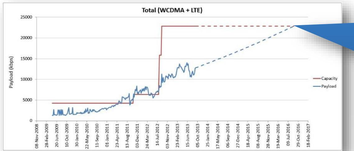
When total WCDMA & LTE payload at this site reaches this level, macro layer spectrum will be exhausted. The operator has knowledge of when more spectrum is required and/or when a micro layer capacity offload solution needs to be implemented.
