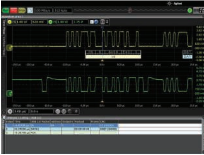
Trigger on and decode USB packets.
