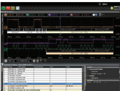
Import BSDL files and decode JTAG scan chain activity.
