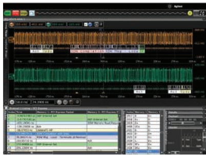
Trigger on and decode PCIe serial packets.
