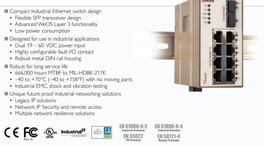
The Lynx 210 is a layer 3 industrial Ethernet switch, powered by the Westermo WeOS network operating system. Lynx is the most compact and has the lowest power requirements in this class of switch. Lynx has 8 10/100 Mbit/s ports in addition to 2 ports which can be fitted with Gbit or 100 Mbit SFP transceivers.
