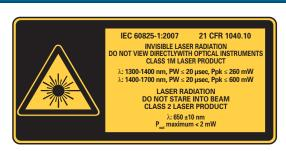
CAUTION: VIEWING THE LASER OUTPUT WITH CERTAIN OPTICAL INSTRUMENTS (FOR EXAMPLE: EYE LOUPES, MAGNIFIERS AND MICROSCOPES) WITHIN A DISTANCE OF 100 MM MAY POSE AN EYE HAZARD.
