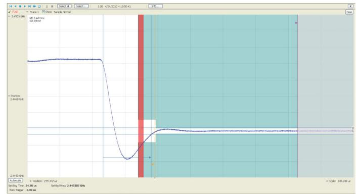
Settling time measurements (Option SVT) are easy and automated. The user can select measurement bandwidth, tolerance bands, reference frequency (auto or manual), and establish up to 3 tolerance bands vs. time for Pass/Fail testing. Settling time may be referenced to external or internal trigger, and from the last settled frequency or phase. In the illustration, frequency settling time for a hopped oscillator is measured from an external trigger point from the device under test.
