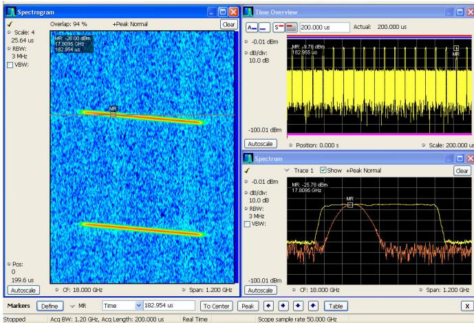
Once captured into memory, SignalVu provides detailed analysis in multiple domains. The spectrogram display (left panel) shows the frequency of an 800 MHz wide LFM pulse changing over time. By selecting the point in time in the spectrogram during the On time of the pulse, the chirp behavior can be seen as it sweeps from low to high (lower right panel).
