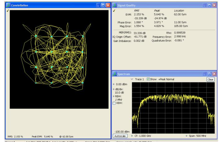
Wideband satellite and point-to-point microwave links can be directly observed with SignalVu analysis software. Here, General Purpose Digital Modulation Analysis (Option SVM) is demodulating a 16QAM backhaul link running at 312.5 MS/s.
