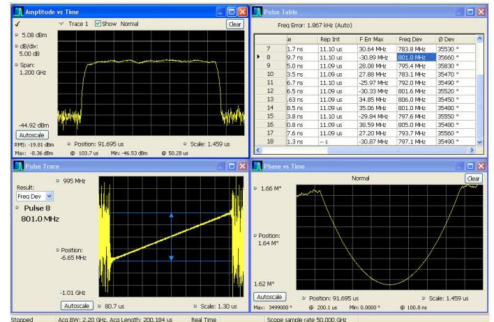
The Advanced Signal Analysis package (Option SVP) provides 27 individual measurements to automatically characterize long pulse trains. An 800 MHz wide LFM chirp centered at 18 GHz is seen here with measurements for pulses 7 through 18 (upper right). The shape of the pulse can be seen in the Amplitude vs. Time plot shown in the upper left. Detailed views of pulse #8's frequency deviation and parabolic phase trajectory are shown in the lower two views.
