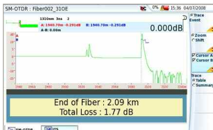
OTDR/fault locator screen
