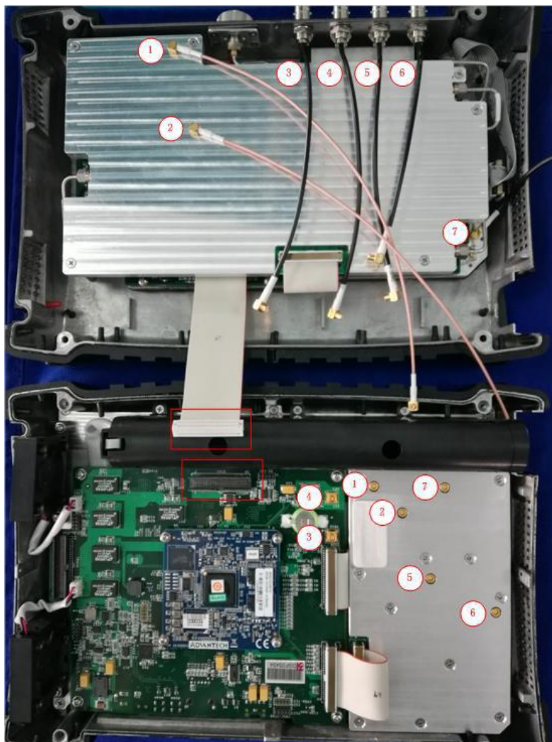
Fig.5 Connection cables between the front and rear casings
