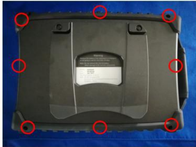
Fig.4 Removal of 6 fixing screws
