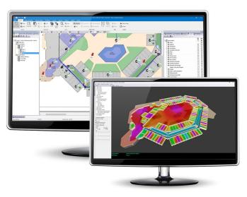
Adjust 3D view layers. In the 3D modeler, you can adjust all planes of your design (x,y,z) to view your building as a whole or floor by floor. You can also adjust visible layers to choose what you are looking at: cabling, APs, network equipment, prediction). Zoom in, walk through and pan your design and export an image to include in reports or send to your customer.
