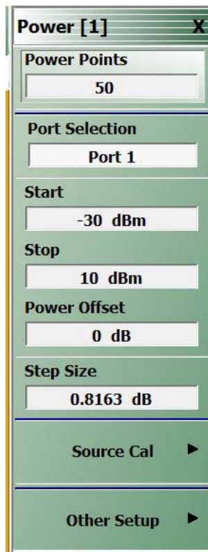
Figure 14-5. Main Power Sweep Menu - POWER [COUPLED] Menu
