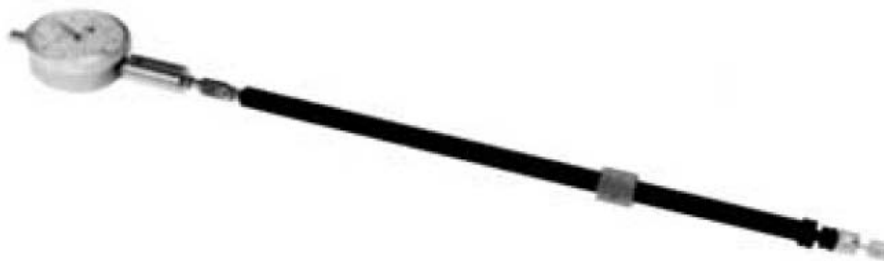
Figure 1-14. F-F Sliding Terminator with Attached Dial Gauge
