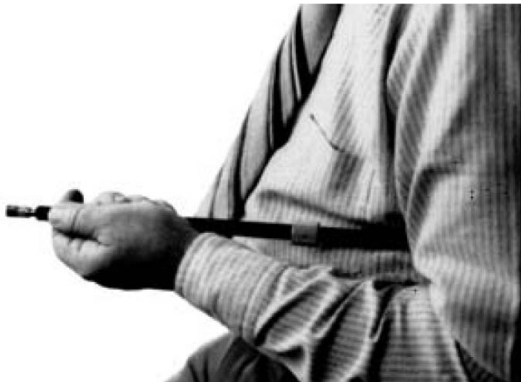
Figure 1-10. Holding F-F Sliding Terminator, Ready to Measure
