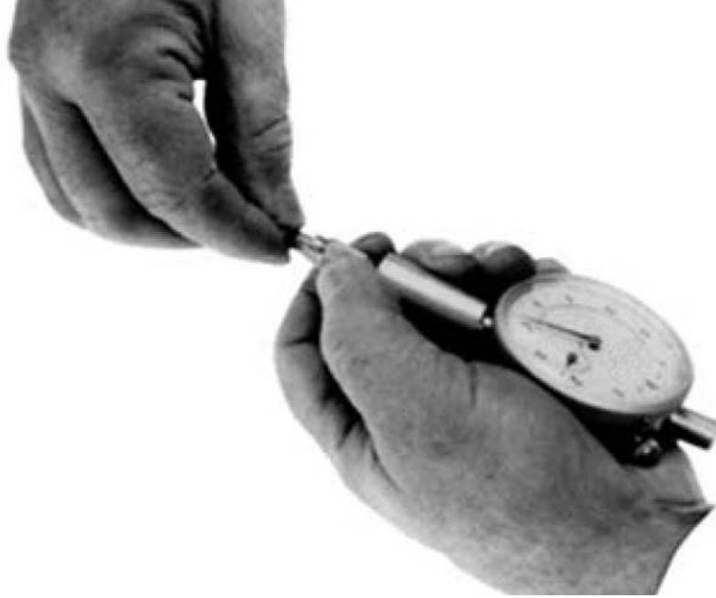
Figure 1-20. Installing the Female Adapter on the Gauge
