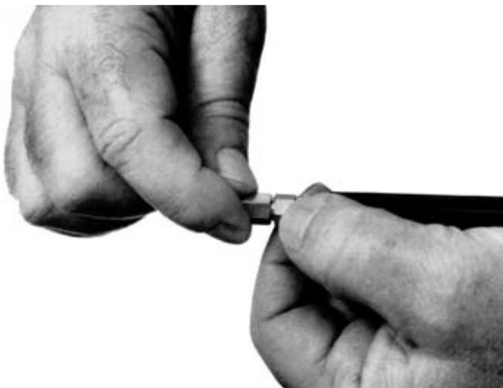
Figure 1-11. F-F Sliding Terminator, Removing Flush Short
