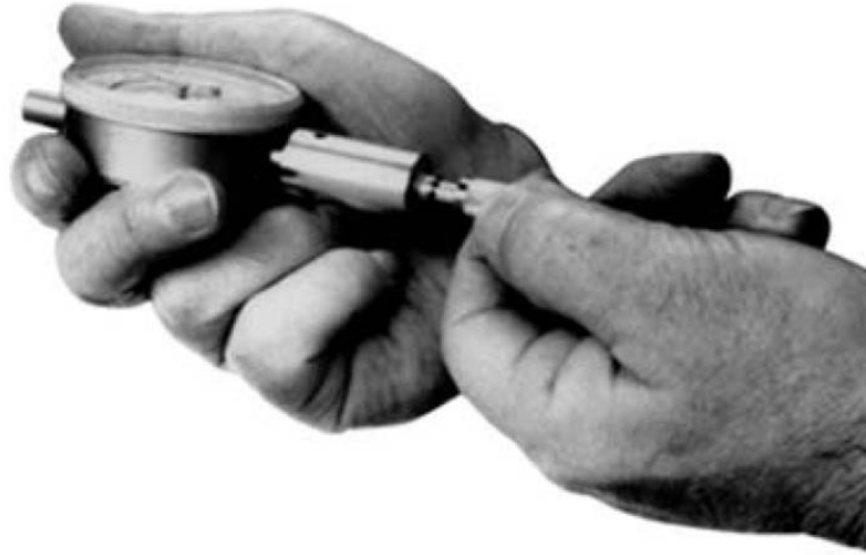
Figure 1-12. F-F Sliding Terminator, Installing Gauge
