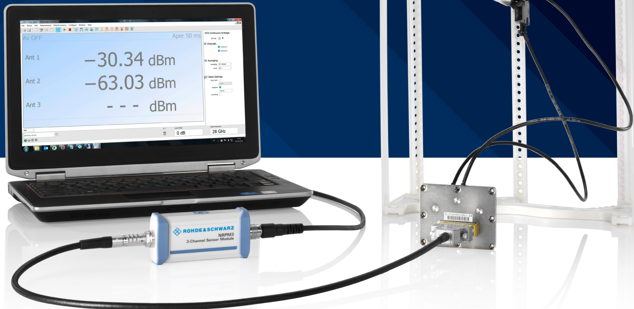
R&S®NRPM OTA power measurement solution with R&S®NRPM-A90D dual-polarized antenna module for use with a shielded RF test box
