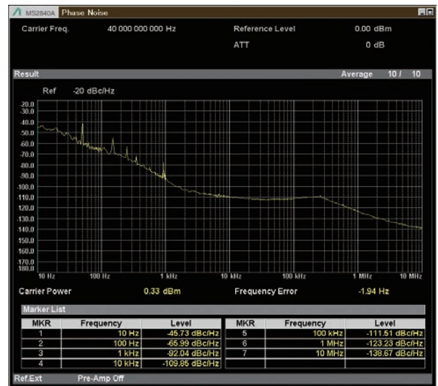
Phase Noise Measurement 40 GHz Measurement Frequency, Preamp Off
