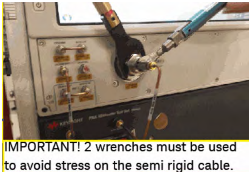
Figure 3-7 To avoid damaging your RF ports 1/2/3/4, always use two wrenches
