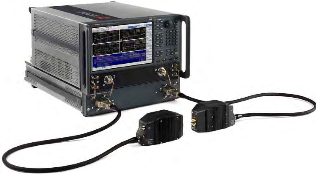
Figure 3-16 Cable Two Test Heads N5293/5AX03 to the N5292A. (Attach heads and torque cable screws to 8 in-lbs.)
