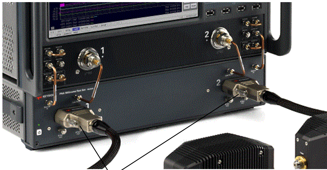
Figure 3-16 Cable Two Test Heads N5293/5AX03 to the N5292A. (Attach heads and torque cable screws to 8 in-lbs.)
