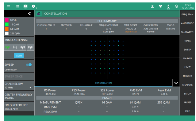
Constellation diagrams of LTE PBCH and PDSCH highlight distortions in transmitter modulators
