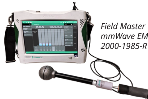
EMF results show power from each antenna axis and summary results for peak and average power over a defined time period
