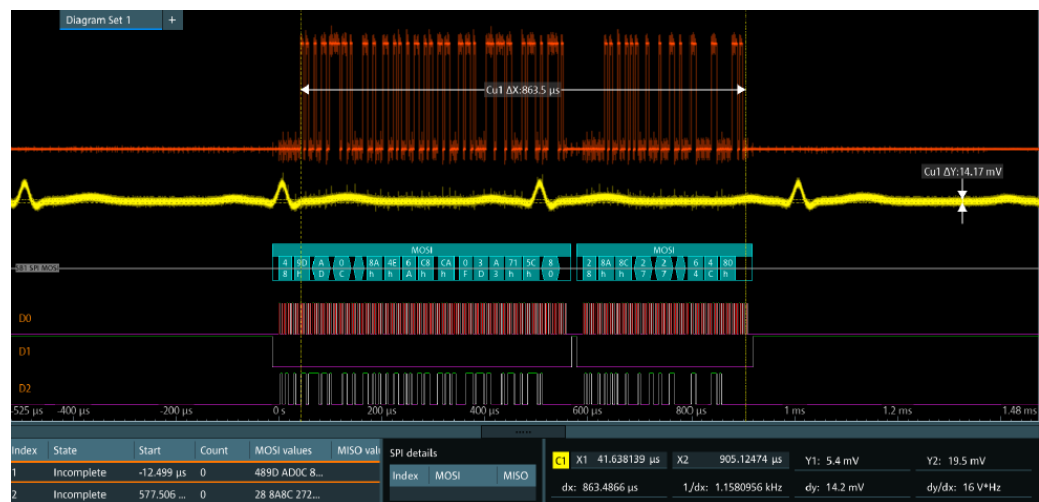
Figure 13-2: Decoded and binary SPI signal
