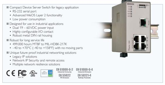
Lynx DSS is available in several versions, the L105-S1 is a device server with a layer 2 industrial Ethernet switch, powered by the Westermo WeOS network operating system. Lynx DSS is the most compact and has the lowest power requirements in this class of device servers. Lynx DSS has 4 10/100 Mbit/s ports and one RS-232 port.
