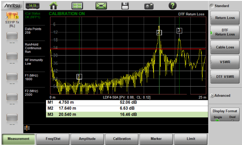
Figure 3-13. DTF Return Loss Measurement (Antenna at 20.54 m)
