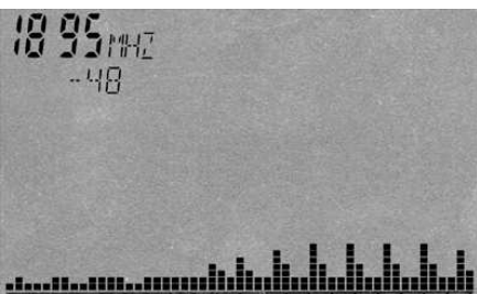
Well visible: "Frequency hopping" of a DECT portable phone between 1890 and 1900 MHz (Screenshot)
