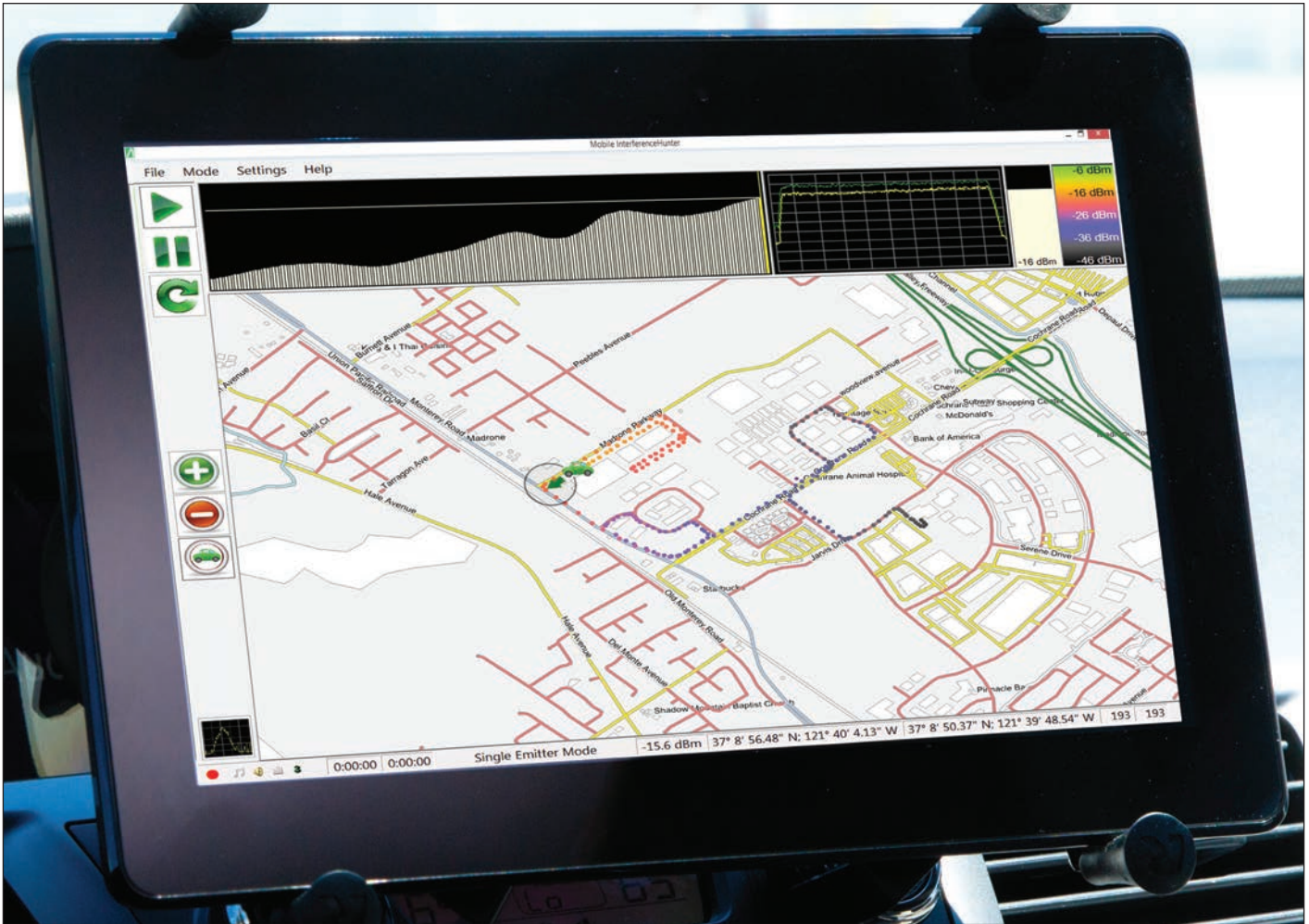
Interference hunt screen capture. Dots shown along drive path are colored according to signal strength.
