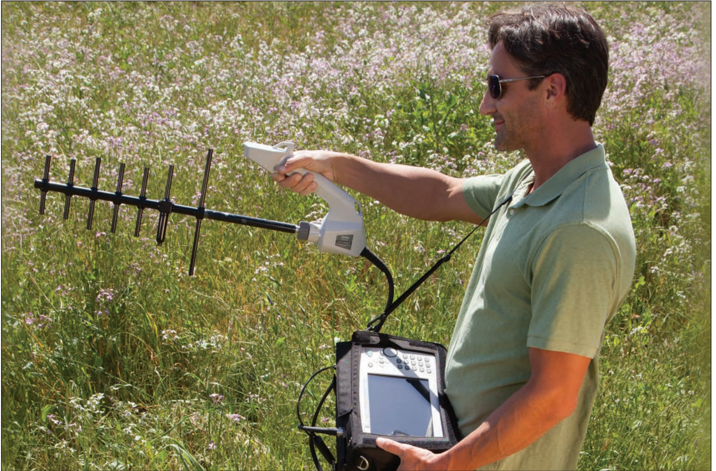
Pinpointing interference location with the MA2700A Handheld IntefereceHunter.
