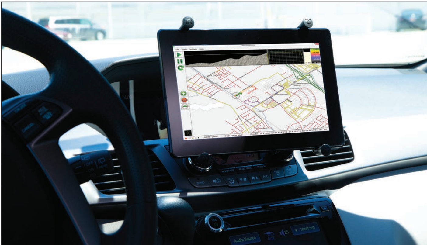
Mobile InterferenceHunter™ on Windows® PC Tablet with Spectrum Master™ in Vehicle
