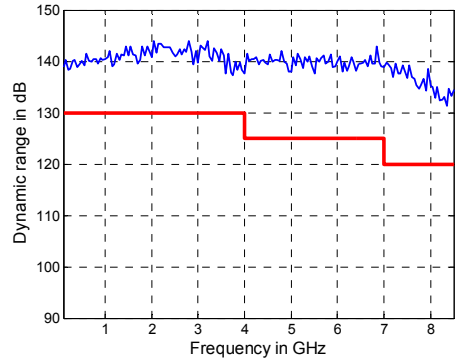
Dynamic range in dB versus frequency for the R&S ® ZNB8.
