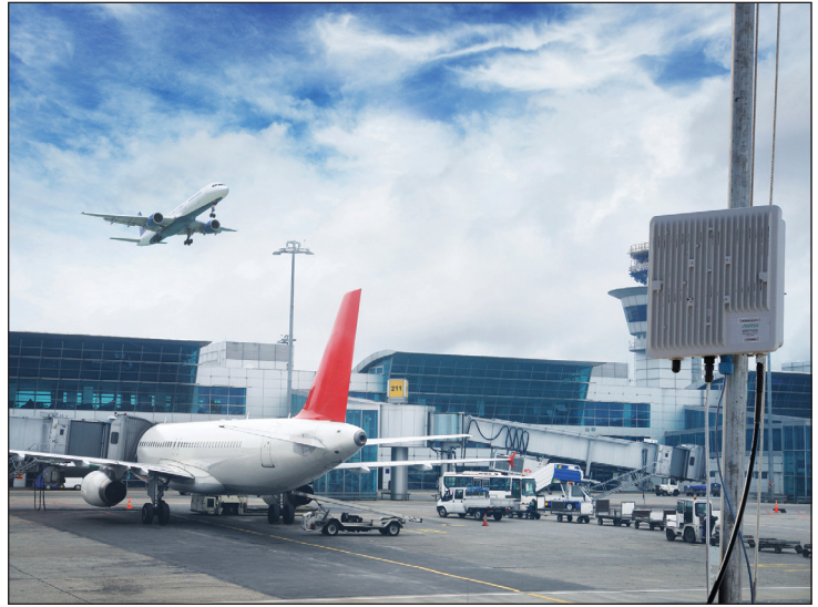
Fig 8: Anritsu remote spectrum monitor positioned at airport
