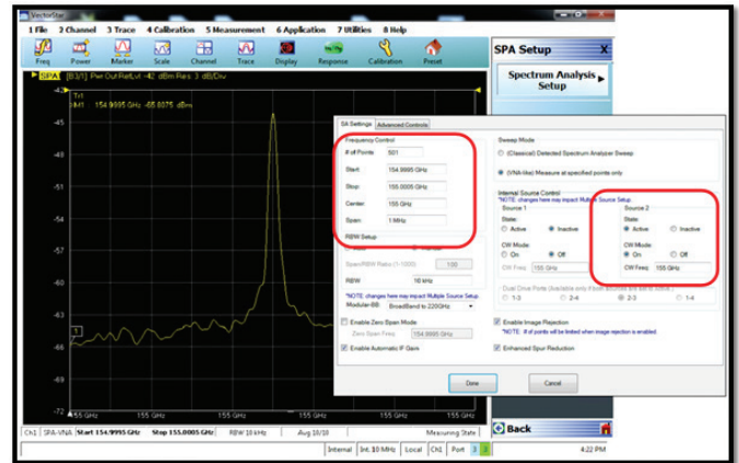
Independent Tracking Control of Sources and Receivers – Showing a 155 GHz Tracking Mode
