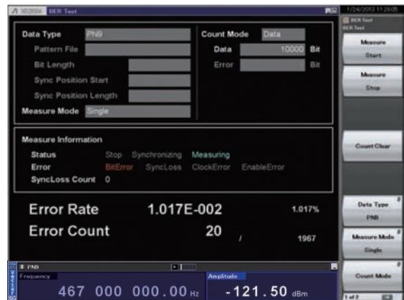
BER Measurement Function (top) and Vector Signal Generator (bottom) Measurement Examples
