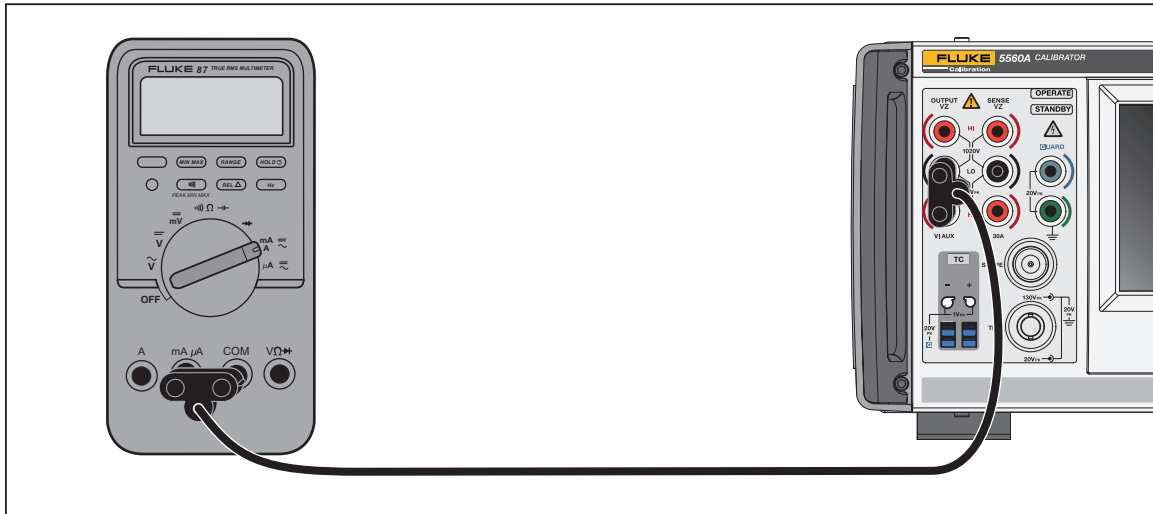
Figure 7. DUT Connection: DC Current/AC Current <3.1 A
