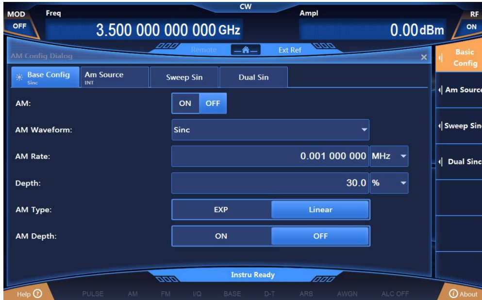
Fig.2.22 Setting of Amplitude-modulated Signals
