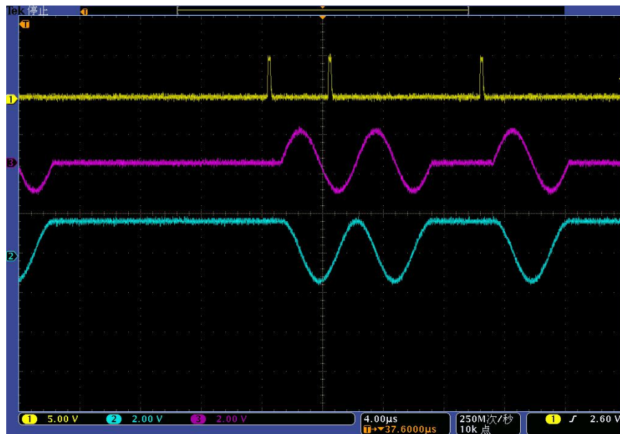
Fig.3.26 Diagram of Arbitrary Trigger (Single/Buffer Repeated Trig)
