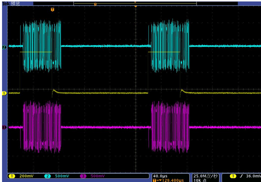
Fig.3.21 Diagram of Baseband Triggering (Continues/Single)
