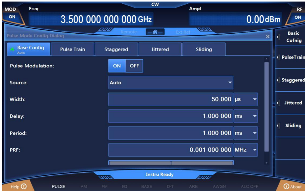
Fig.2.23 Setting of Pulse-modulated Signals
