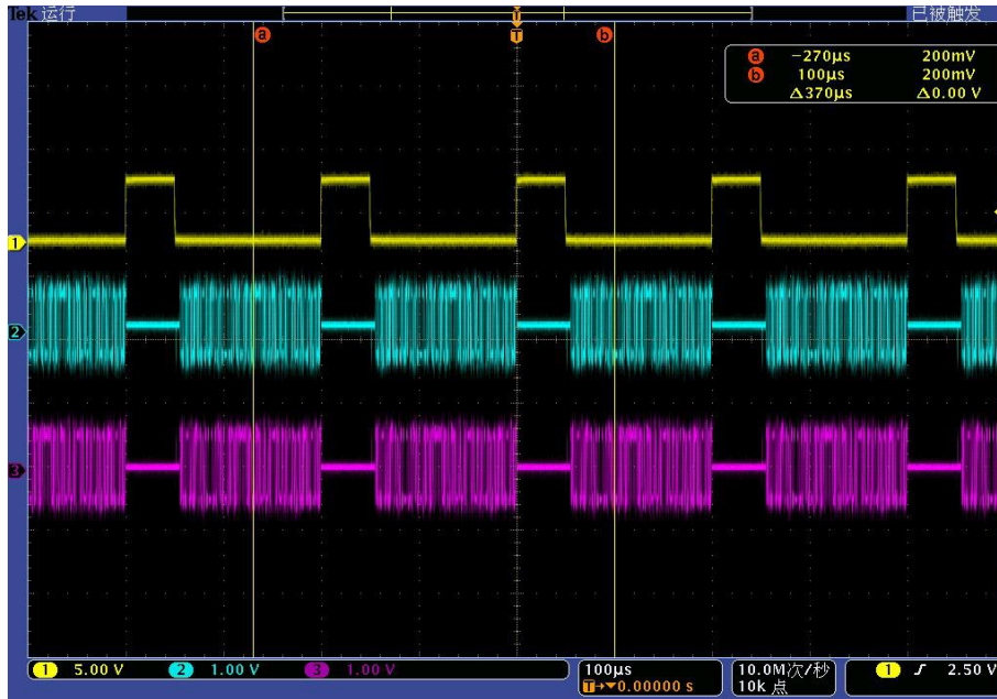
Fig.3.23 Diagram of Baseband Triggering (Gate/Low)
