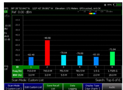
Scan up to 20 channel simultaneously with the channel scanner option
