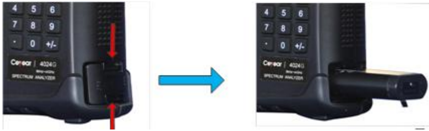
Fig. 2 Removal of Battery
