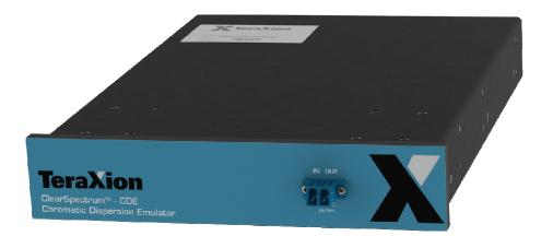
This 1U half 19-inch rack mountable module is designed to emulate tens of thousands of picoseconds per nanometer in a compact unit while maintaining very low insertion loss. Entirely passive, it can be cascaded several times to achieve the desired dispersion level.
