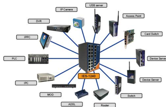
Connections of Ethernet devices
