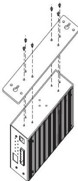
2. Use the switch, with wall mount plates attached, as a guide to mark the correct locations of the four screws.
