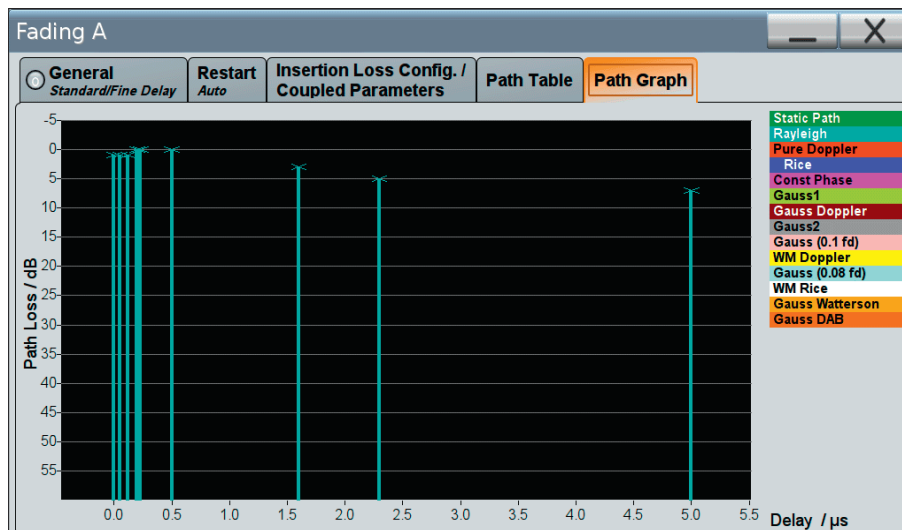
The fading settings of the R&S®SMW200A can be visualized to support the user. The screenshot shows the fading path configuration of an LTE ETU300 scenario.
