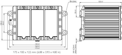
Weight 2.2 kg Degree of protection IP 40
