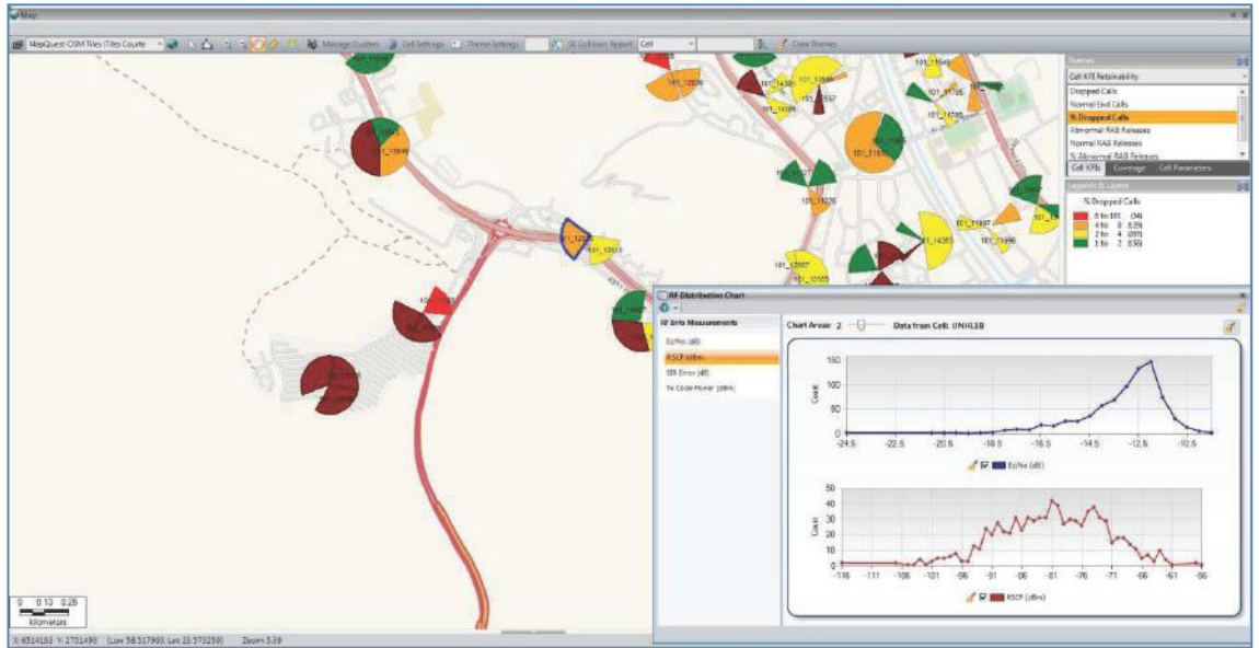
Figure 35 - Investigating cells with high dropped call number, also showing RF Distribution Chart for poorly performing cell
