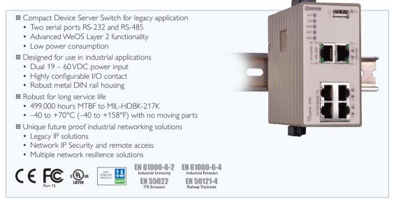
Lynx DSS is available in several versions, the L106-S2 is a device server with a layer 2 industrial Ethernet switch, powered by the Westermo WeOS network operating system. Lynx DSS is the most compact and has the lowest power requirements in this class of device servers. Lynx DSS has 4 10/100 Mbit/s ports and two serial ports. One of the serial ports is configured for RS-232 the other one can be configured for RS-232 or RS-422/485.
