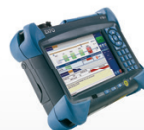
Platform FTB-720 QUAD OTDR/iOLM
