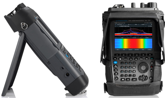
The R&S®PR200 has a fold-out support for desk top use and also the R&S®HA-Z22 carrying with sun shade.
