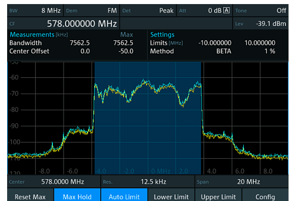
Automatic occupied bandwidth measurement of a DVB-T signal (β % method).
