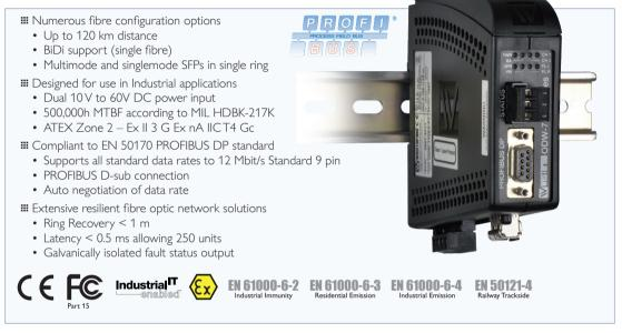
The ODW-710-F1 EX is an ATEX certified PROFIBUS modem that has been designed to allow the use of fibre optic cables on PROFIBUS DP networks. The design allows the use of a range of Westermo verified SFP (Small Form Pluggable) transceivers which can provide solutions with, for example, only a single fibre or distances up to 120 km. Both multidrop networks and redundant rings can be formed using a mixture of transceiver types.
