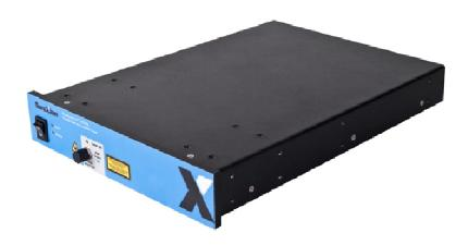
The PS-TNL is an ITLA based, C-band tunable, narrow-linewidth laser source, featuring optical filtering of white frequency noise by an ultra narrowband multi-wavelengths Fiber Bragg Grating (FBG), optimized for coherent communications research.
