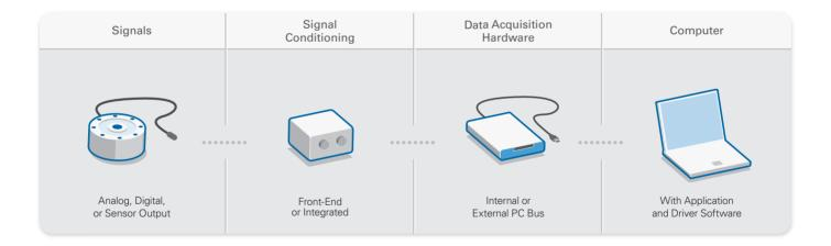
You can use data acquisition tools for a variety of applications such as data logging, control, test automation, monitoring, and prototyping. Use NI data acquisition (DAQ) to meet application challenges for any signal on any bus with easy, powerful software.
