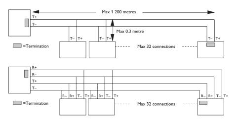
**N.B.** R+/R-,T+/T- definitions are not standard, it can help to shift + and - if the unit does not work.
