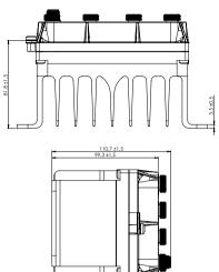
Weight 1.7 kg Degree of protection IP67
